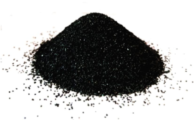
This steel grit is spherical, with high carbon content. Perfectly controlled heat treatments give it optimum resistance to fatigue and resilience. It is suitable for the shot peening and other similar applications. Unlike shot, steel grit is more aggressive. It is commonly used in various industries and has a higher bulk density. It is available in various sizes and is ideal for cleaning surfaces.
